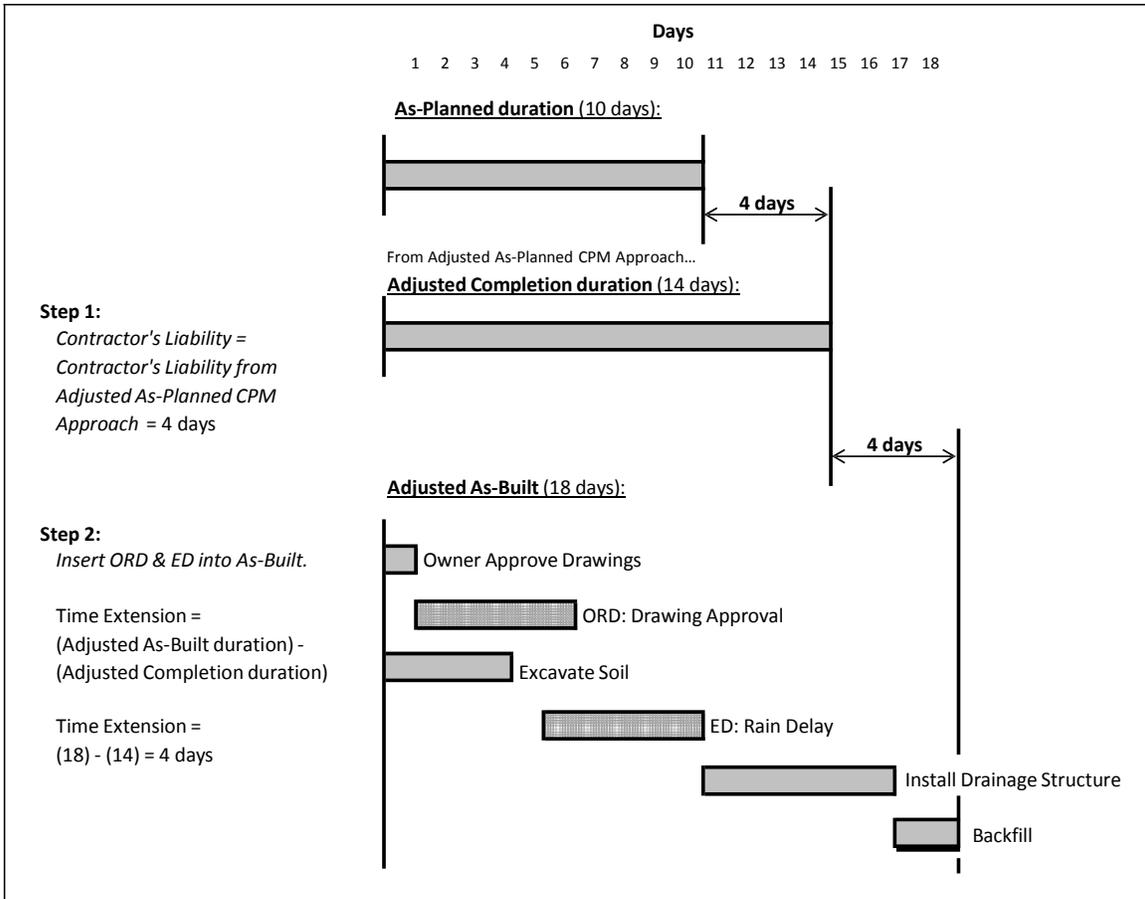
**Figure 17: Adjusted As-Built CPM Approach**
