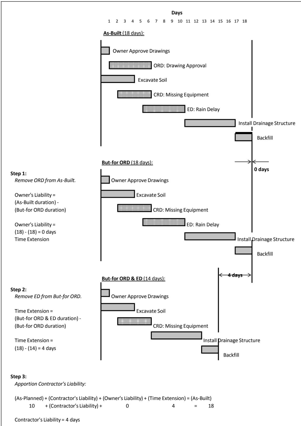
**Figure 18: Collapsed As-Built Schedule (But-for) Approach**
